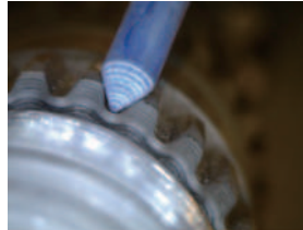
Meister Finish Rod type customized to deburr a rounded groove in a spline.
