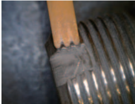
Meister Finish Stick type customized to deburr a key groove in a thread.
