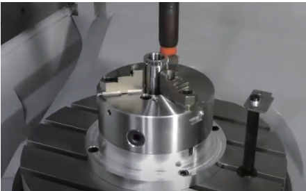
Self-adjusting sleeve in use
