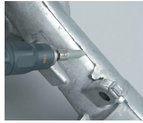
Material: Aluminum Tool: AX-PM-6T
